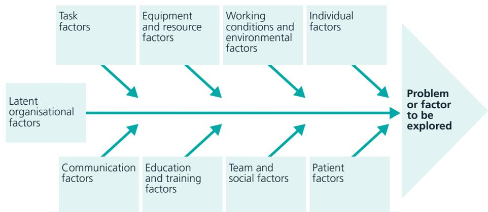
A way of representing contributory factor information is the fishbone diagram or cause and effect diagram. A common approach is to draw a horizontal arrow on a large sheet of paper or white board. Note down the issue or problem to be explored at the head of the arrow. Then add spines to the arrow in a fishbone arrangement, giving each spine a classification heading (from the NPSA contributory factors outlined in Step 1 and repeated below for ease of reference). These
